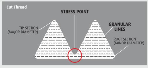
Granular lines of a cut thread are completely cut through leaving the threaded roots (minor diameter) exposed as high stress points for tensile stress buildup.
