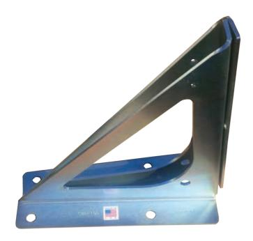
This new bracket system is designed for lower cost and easier installation of smaller shade sails on wood decks or concrete patios. Using a locally sourced 4" x 4" or 4" x 6" wooden post and eye bolt, this system will enable the customer to install cantilevered attachments without the need for digging holes or pouring concrete footing. Will also fit metal posts or round posts. Engineering report is available—ask your Polyfab distributor.
