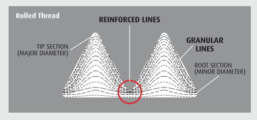
Granular lines are not broken but enhanced in the tip section (major diameter) and root section (minor diameter) of a rolled thread process, making a rolled thread resistance to fatique before tensile stress can be formed.
