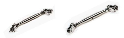
It is recommended that an anti seize product be used on turnbuckle threads to minimize binding.
